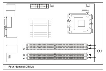
Figure B-21. Four Identical DIMMs
